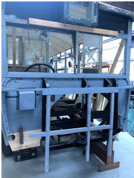
The front end of Ipswich 26 following reframing. [Paul Chandler]
