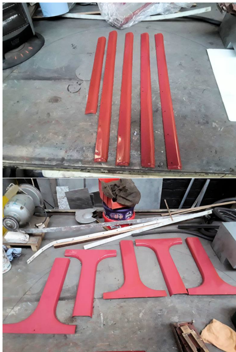
Internal metal window trims for Cardiff 243 being painted in red oxide undercoat.
