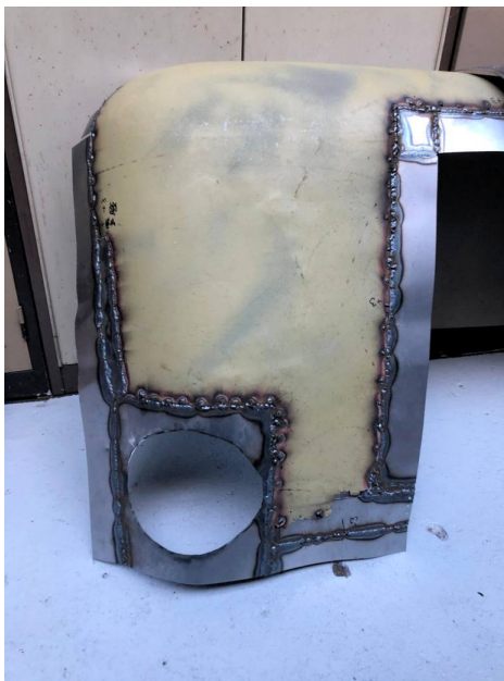
No. 26's front tinware, which will fit over the framework seen in the previous photograph [Paul Chandler]
